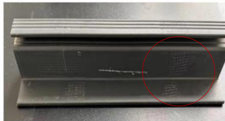
GFRP paint adhesion testing results after salt spray resistance test
